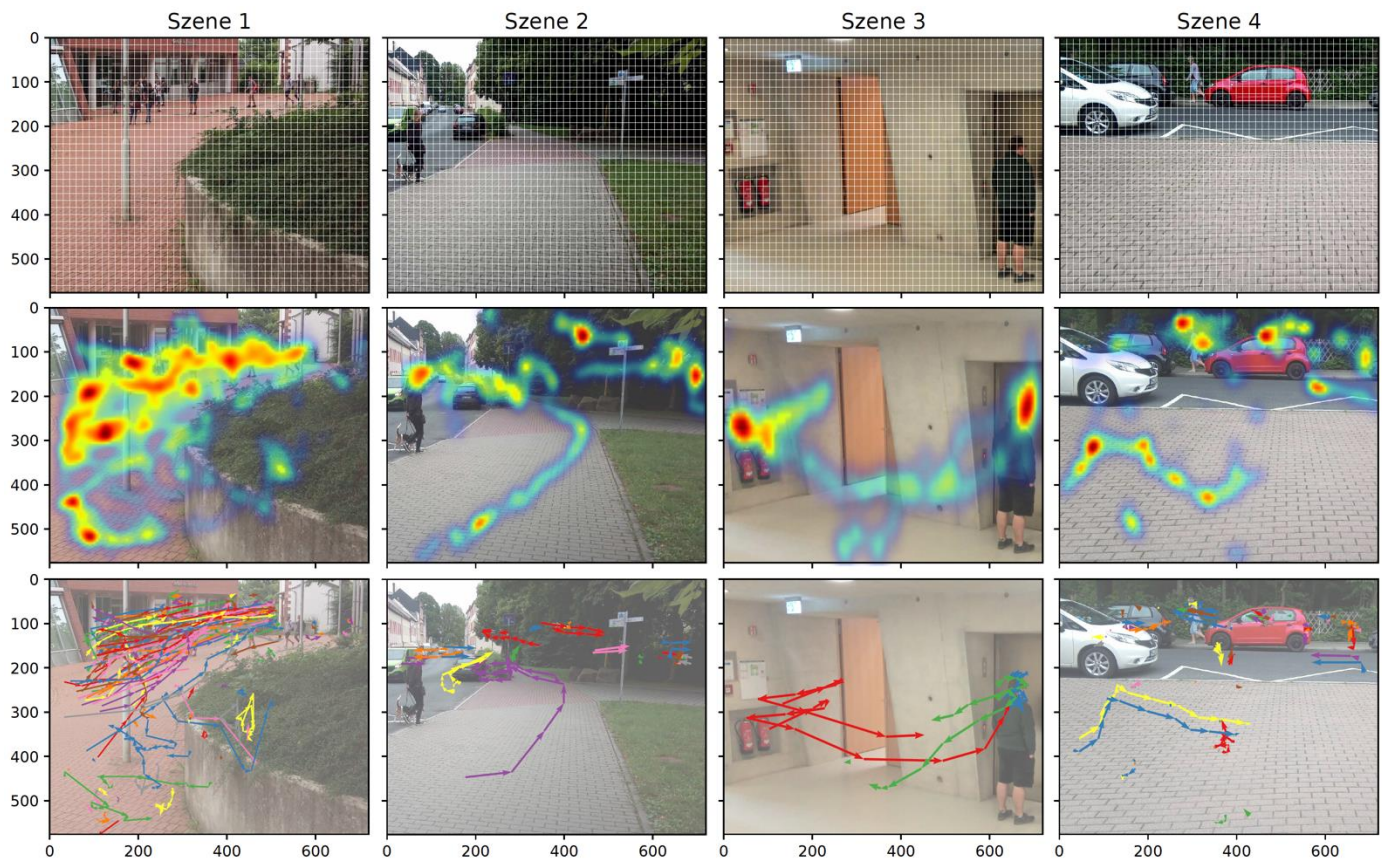
Figure 9: Aggregated visualization of all movements during the runtime of the respective video. Line 1 shows the grid for the heatmap following in line 2, line 3 the vectorized representation.
